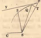
d. area  $= \frac{\ell^2 d \theta}{2}$ ,  $(\theta = \angle C S P)$ , for d. area  $= \frac{Q T \cdot S P}{2}$ .
